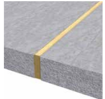
❸ Finished condition of the joint using Plakafeu strips.
