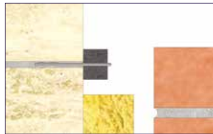
Incorporating U-shaped holder in brickwork joints
