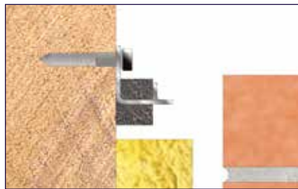
Attaching with wood screw
